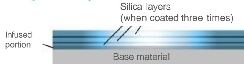
With chemical reaction it fuses silica with the base material to form a strong glass film layer. Therefore, it does not cause cracking, peel-off, deterioration, etc., even if it is coated multiple times. This protects the coated objects for a long time, both functionally and aesthetically.
