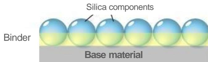
In order to fix silica (glass component) organic binder (adhesive) is used. This organic binder causes deterioration and peeling (Varies by environmental conditions).
